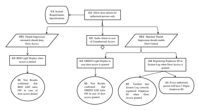
Fig. 2 Assurance Case for Door Access Control Software
